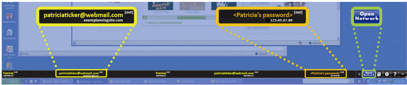
Figure 1. The Ticker display sits above the user’s task bar. The call-outs show some of the terms and indicators that are currently visible; from left to right: Watch List term, “patriciaticker@webmail.com,” was sent out in the clear by “eventplanningsite.com,” and “<Patricia’s password>” was sent out in the clear by IP address “123.45.67.89;” the Wi-Fi Network Status Indicator reflects that the user is currently connected to an “Open Network.”
