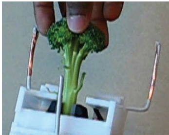
Fig. 10: Basic grasping after 1D alignment: the planar robot used the E-Field sensors to align itself with the target object before attempting the grasp.
