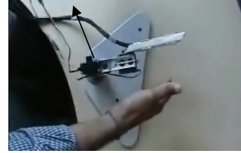
Fig. 6: Human hand avoidance experiment. As the human hand approaches the robot arm, the robot arm moves away.
