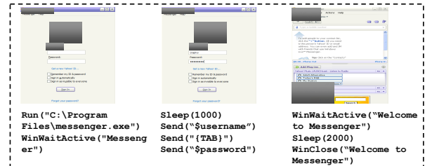
Figure 3: AutoIT script example for testing a popular Internet messenger client. The application is executed in a virtual machine (dotted box)
