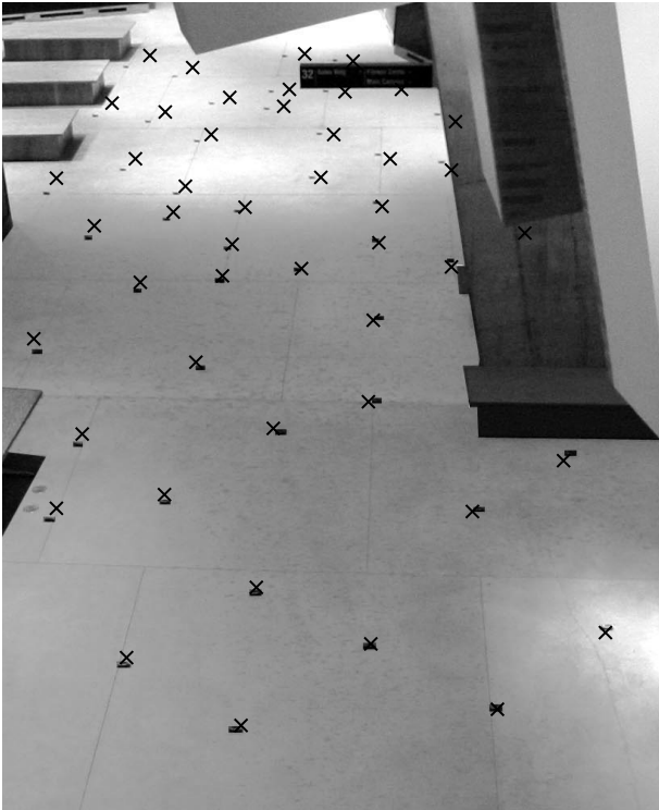
Figure 2: LaSLAT localization result on a sparser sensor network with 49 nodes in a 10m by 17m environment. Crosses indicate the recovered sensor locations, projected onto the image. The average localization error was 7.5 cm.
